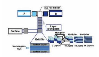
Fabricating biologically inspired gradient index optics involves co-extruding two polymers, A and B, in subwavelength nanolayers that make up 50-µm-thick films. These films form the basis for lightweight, inexpensive gradient index optics. Courtesy of Guy Beadie, US Naval Research Laboratory.
