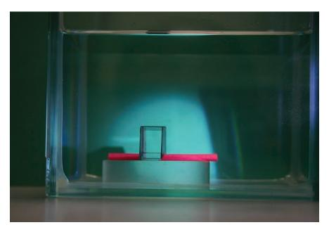
Invisibility through anisotropy: A rolled-up piece of paper sits under a cloak wedge made of calcite, a material with direction-dependent optical properties. The portion of the object inside the wedge is not visible, and the wedge surface appears to be flat, creating a cloaking effect. Courtesy of Baile Zhang and George Barbastathis, SMART Centre, Singapore.
